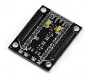
Imagen IV.26: XBee Explorer Regulated
