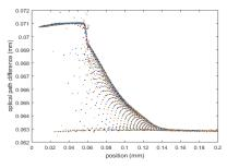
**Conclusion:** The low coherence interferometry technique presented here offers the possibility of studying time resolved capillary filling phenomena with high spatial resolution. The results indicate that the filling dynamics in nanoporous silicon follows a typical Washburn behavior ( $x \propto t^{1/2}$ ). A pronounced widening of the advancing front is condensed into a master curve that only depends on position and could provide valuable information about the morphology of the PS structure.
