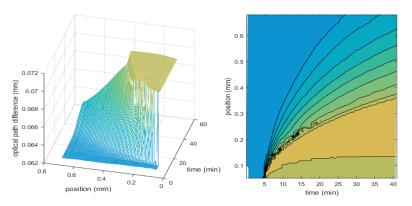
If the optical profiles are normalized to the root of the evolution time all measurements collapse to a single master curve (see figure below) indicating that the liquid front broadening is proportional to the front position. This information can be useful to determine the porous distribution of the PS layer.
