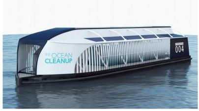
It collects energy by means of solar panels and store energy in lithium batteries. These batteries allow you to operate continuously day and night autonomously. Intelligent on-board software monitors system performance, energy use and component status.
