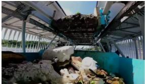
**4. "Dumpsters:** The Interceptor can store up to 50m³ of trash before needing to be emptied. This means it is capable of operating even in the most polluted rivers all over the world."
