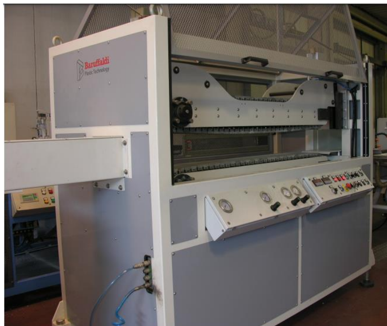
Picture of our haul off type TRAXI 1.5/P ready for delivery
