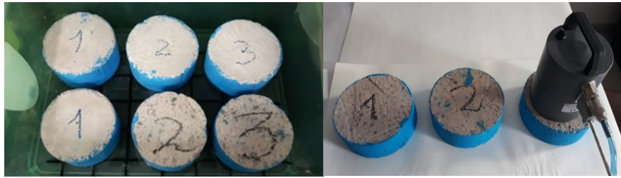
a) b) Fig. 2 Provision of specimens for suction test (a) and air permeability test (b).
