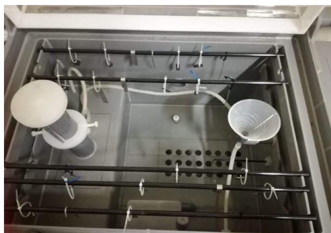
Figure 1. Samples arrangement into salt spray chamber.
