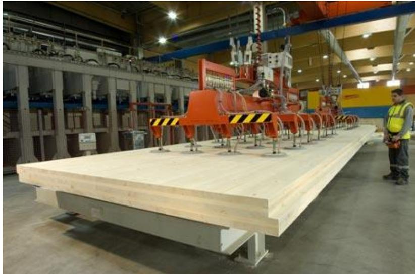
Figura 22: Manufactura de panel CLT.
