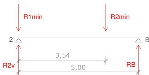
$$\left. \begin{aligned} \Sigma Fv &= -Rv2 - RB + 3,01 t + 1,50 t = 0 \\ \Sigma M2 &= 1,50 t * 3,64 m - RB * 5 m = 0 \end{aligned} \right\} \begin{aligned} RB &= 1,06 \\ R2v &= 3,45 \end{aligned}$$
