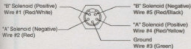
5-Pin Manaplug (Mini) with Lights Single and Double Solenoid Valves
