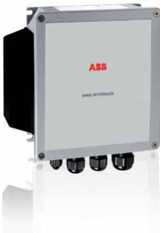
The 4000/7200-WIND-INTERFACE rectifies and filters the alternating current, thus producing a direct current output to feed ABB small wind turbine inverters. This device is suitable for turbines that produce 20 A current maximum.
