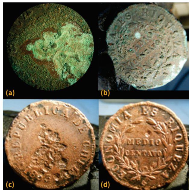
Fig. 1 — The 1853 copper coin before (a and b) and after (c and d) electrolytic cleaning.
