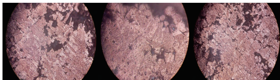
Fig. 4 — Micrograph of the 1853 historical copper coin showing corrosion from pitting. Reagent: Alcoholic solution of 2% ferric chloride ( \text{FeCl}_3 ). Magnification: 100x.
