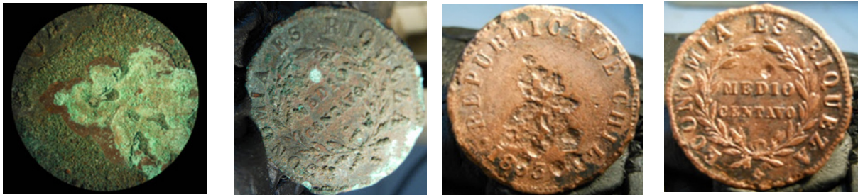
Fig. 5 The before (5 a. and 5 b.) and after (5 c. and 5 d.) of the 1853 historical copper coin to electrolytic cleaning and macroscopic images.
