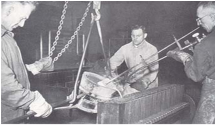
Fig. 13 The molten metal was poured into the rail, with moulds in the shape of ingots
