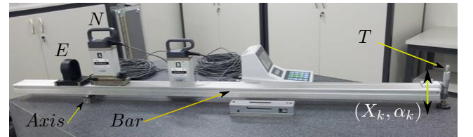
Fig. 6: Experience with electronic level and autocollimator.
