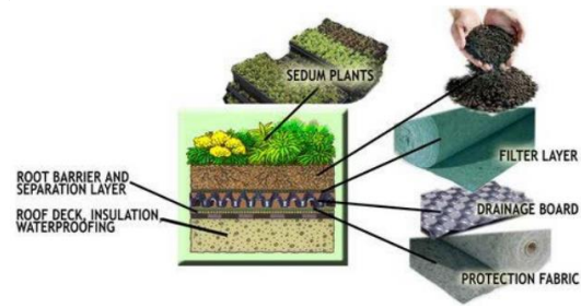
Fig. 2. Extensive green roof [8, pp. 3]
