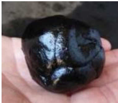
Fig.11. Appearance of CA20 binder modified with recycled plastic
