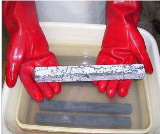
FIGURE 4: Cracking in mortar bar
