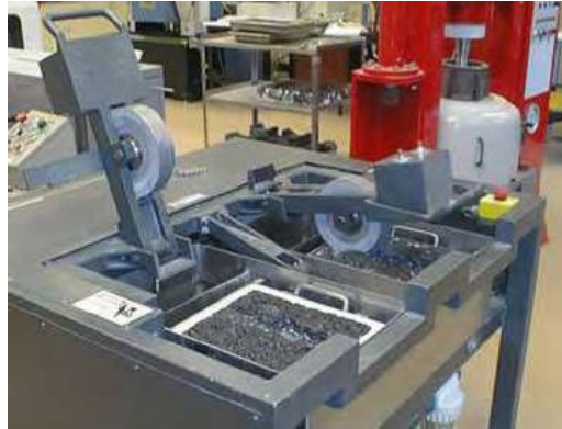
Figura 3.20. Hamburgo Wheel Tracking Device (HWTM). (Delbono, 2014)
