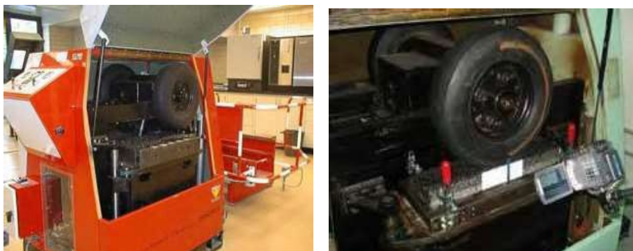
Figura 3.19. Probador Pavement Rutting (LCPC). (Delbono, 2014)
