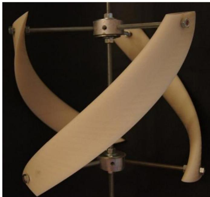
Figure 3.11. Model 3 bladed, NACA 0022 profile, 55% solidity turbine
