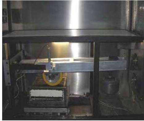
Figura 3.22. Wheel Tracking Test (WTT). (Delbono, 2014)
