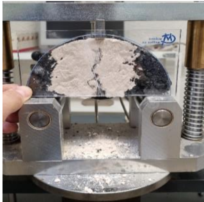
Figure 9: Crack propagation test by bending test of a semicircular specimen.
