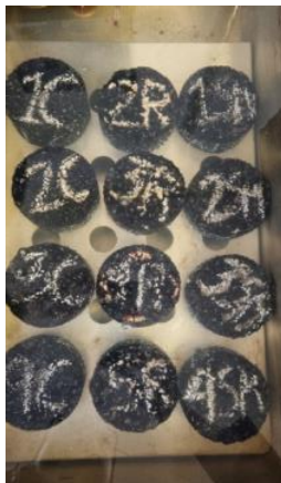
Figure 7: Water sensitivity test: Conditioning and testing.
