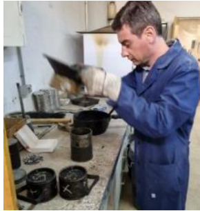
Figure 5: Mold filling and Marshall compaction.
