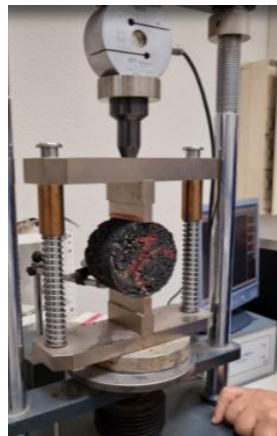
Figure 7: Water sensitivity test: Conditioning and testing.
