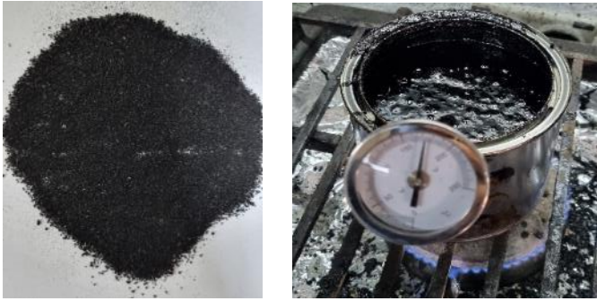
Figure 1: Left: NFU; Right: manual pre-mix asphalt-NFU.
