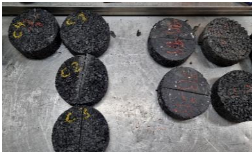
Figure 6: Production of semicircular specimens.
