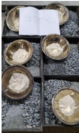
Figure 4: Preparation of aggregates for Marshall specimens.
