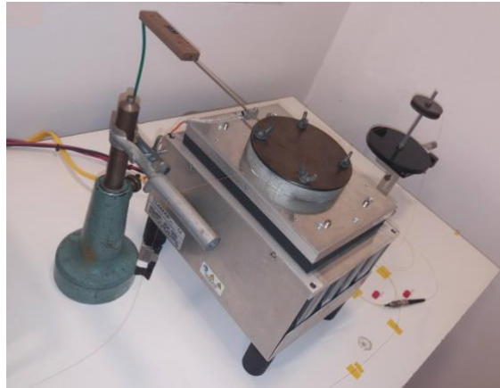
Fig. 14. Temperature sweep performed to determine thermal sensitivity.
