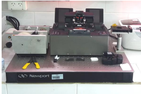
Fig. 7. Experimental setup for LPG fabrication. Physical implementation.
