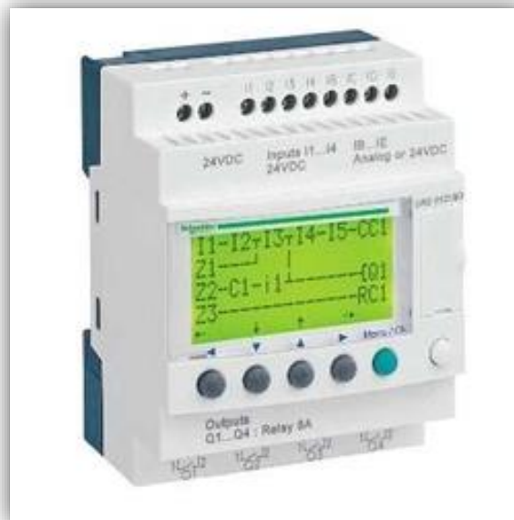
Fig. 1 Smart Relay. Tomada de [1]
