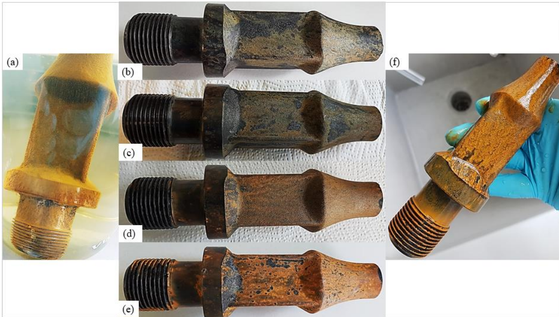
Fig. 4.2 - (a) Rod in-water after 6 days; (b) Dried rod after 7 days; (c) Dried rod after 8 days; (d) Dried rod after 15 days; (e) Dried rod after 26 days; (f) Recently removed rod after 15 days.
