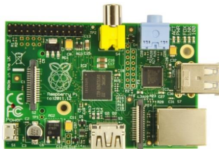
Figura 44 –Raspberry 1 model B
