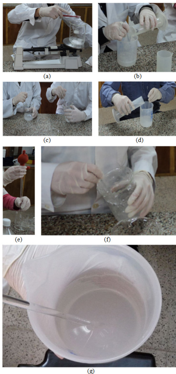
Figure 3. (a) Measurement of carbopol, (b) Added of distilled water, (c) Stirring, (d) Added of ethyl alcohol 96 %, (e) Added glycerin, triethanolamine and essential oil, (f) Stirring, (f) Gel alcohol
