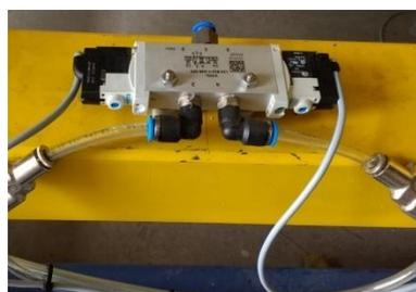
**Fig.Num°49:** Válvula FESTO vuvg-l14-b52-t-g18-1p3.
