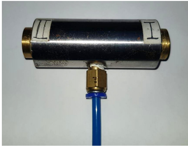
Fig. 7 Hollow object employed to measure the microdeformations experienced by its end faces when applying pneumatic pressure inside it.
