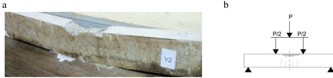
Figure 6. (a) Failure of the control beam and (b) schematic drawing.
