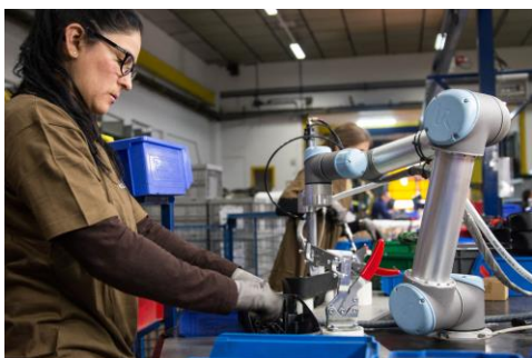
Fig. 3. A collaborative robot assisting an operator in an assembly task. Source: https://blog.universal-robots.com/es/industria-40
