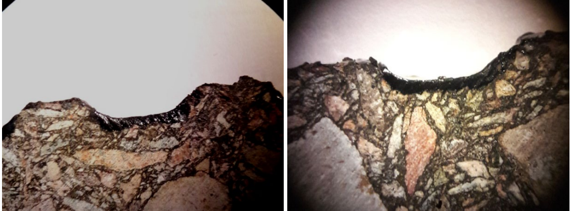
Figure 8. Disposition of tack coat achieved in laboratory
