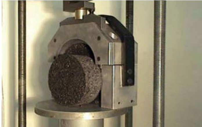
Figure 2. Shear bond test (SBT) (Montetrusque et al. 2015)
