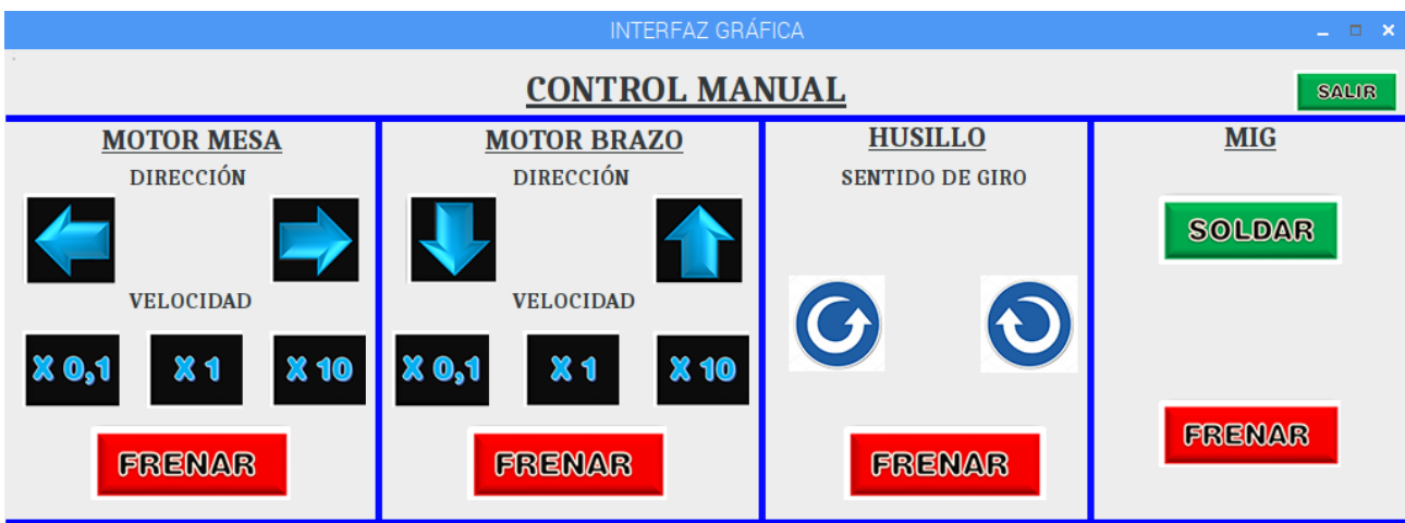
Figura 18: HMI control manual.
