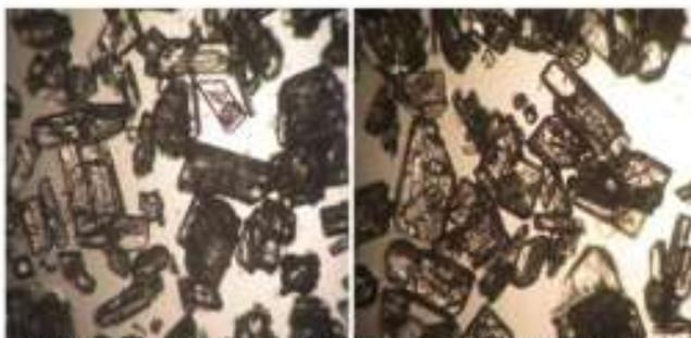
Fig. 12: Microscopic Graphs of Potassium Sulfate Crystals Obtained by Applying the Recommended Operating Parameters.
