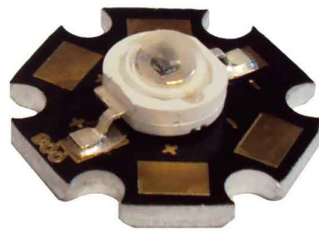
Figura 13. Led High Power 3W infrarrojo de 850nm [36].
