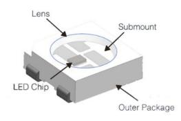
Figure 2: UV-C LED Structure [1]
