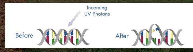
Figure 1: UV Disinfection Process [1]
