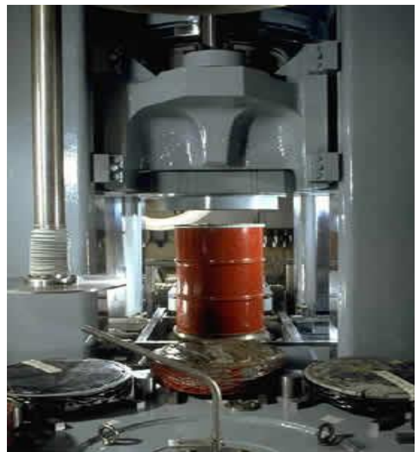
Fig. 2. The process of compaction [6]
