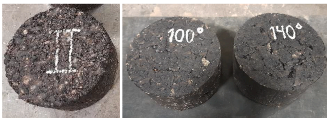
Fig. 7. Specimens moulded with the test mixture, a) Group (1) and b) Groups (2) and (3).
