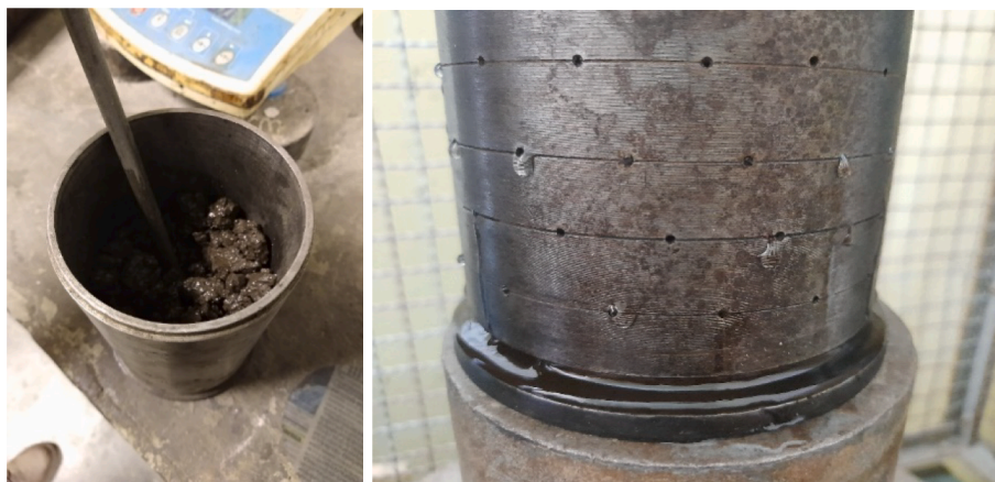
Fig. 6. a) placement of the mixture in the mould and b) specimen compaction.
